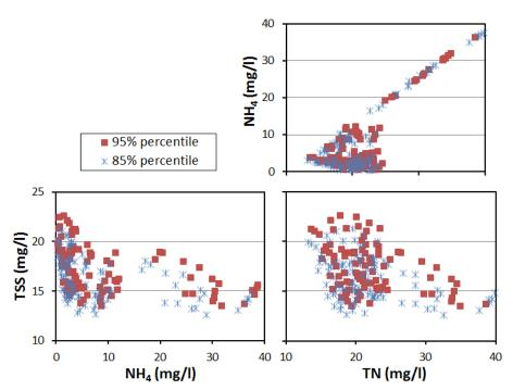
**Figure 6**. Relationships between the output variables expressed as 95% and 85% percentiles of the average values of NH<sub>4</sub>, TN and TSS in the effluent.
