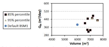
**Figure 7**. Relationship of the volumes and waste flow rates of the designs that fulfil the effluent requirements with a 95% and 85% probability of compliance
