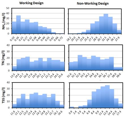
**Figure 4.** Histograms of the average values of NH<sub>4</sub>, TN and TSS in the effluent for a Working Design (WD) and a Non-Working Design (NWD).
