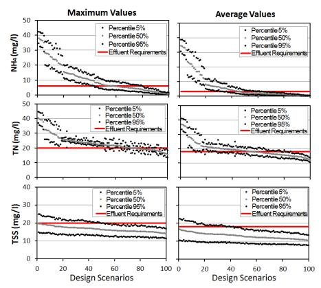
**Figure 5**. Median and 90% percentiles of the maximum and average values of the NH<sub>4</sub>, TN and TSS effluent concentrations for 100 plant designs.
