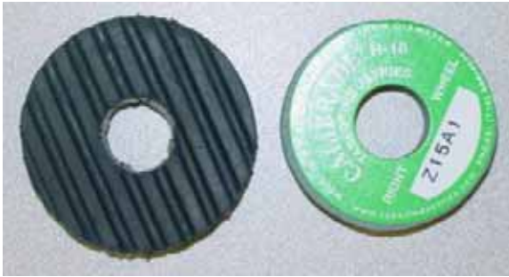
Figure 4.23 Image of composite rubber belt wheel (left) cut from V-belt material, used on Modified Taber Test Stand.
