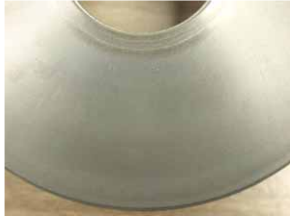
Figure 4.20 Image of the Hardcoat anodized movable sheave.
