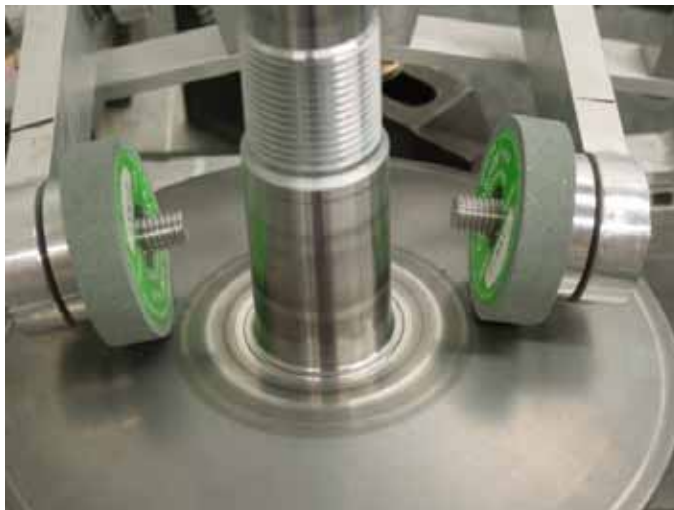
Figure 4.14 Figure showing abrasion test stand based off the Taber Abraser design. The two arms were at the same angle as the sheave surface allowing the wheels to rest normal to the surface.
