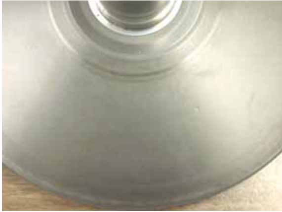
Figure 4.19 Image of the Hardcoat anodized stationary sheave.
