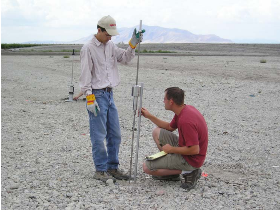
FIGURE 3-9 Dynamic cone penetrometer.
