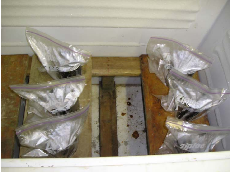
FIGURE 3-7 Freeze-thaw specimens in freezer.
