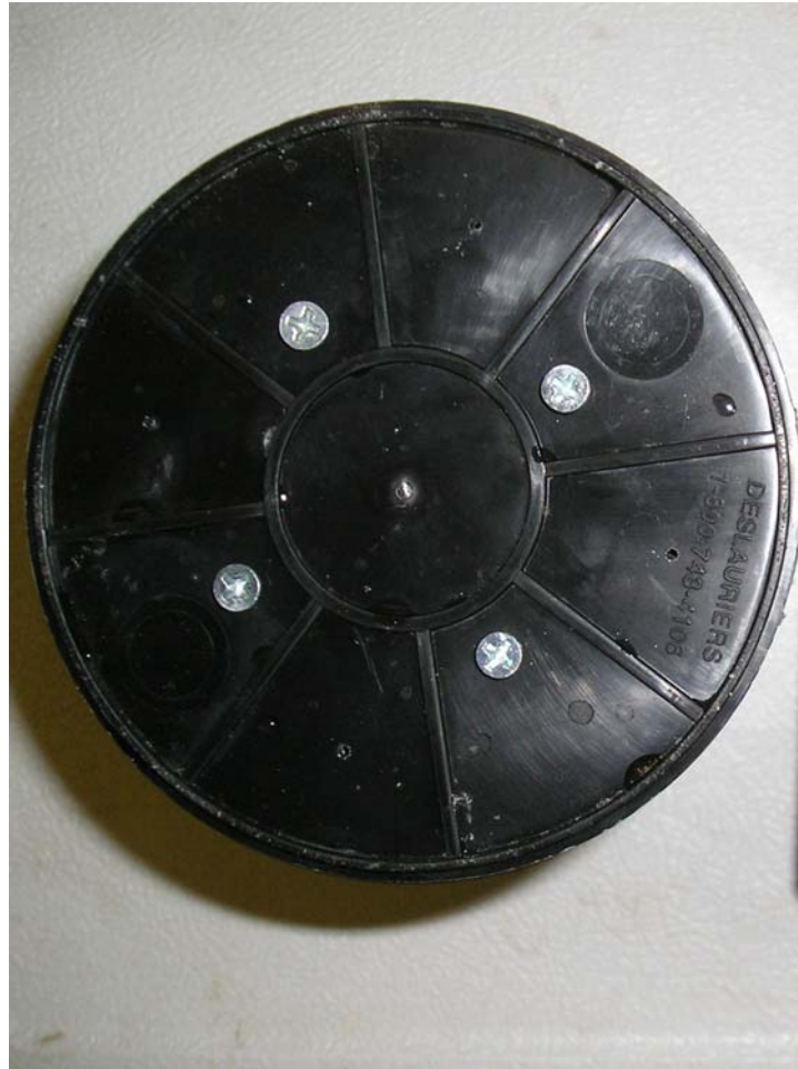
FIGURE 3-4 Specimen mold for stiffness testing.
