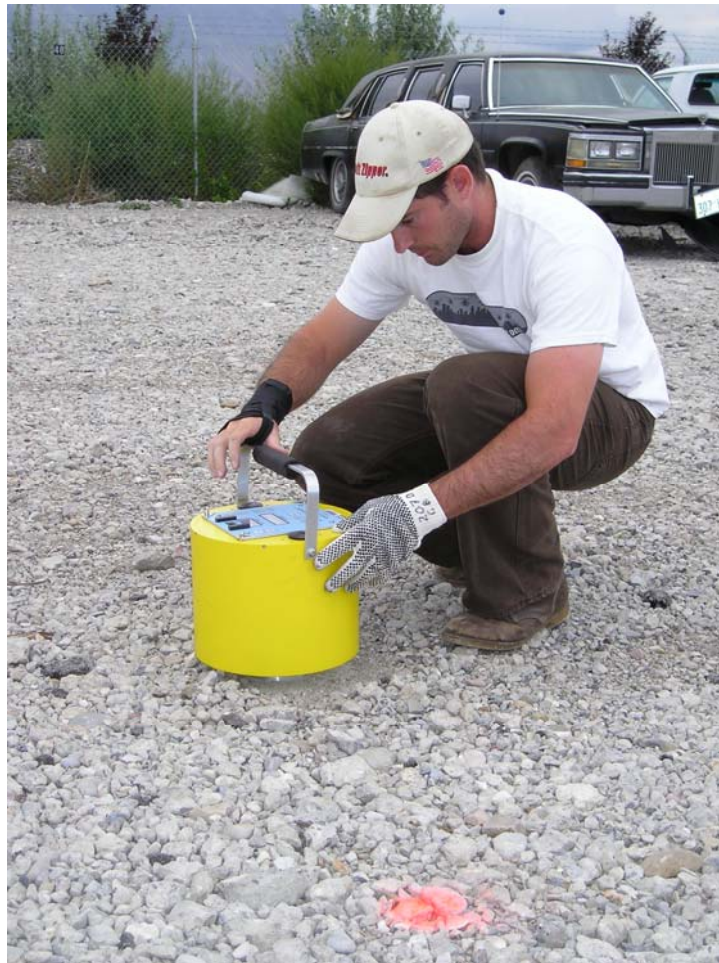
FIGURE 3-12 Soil stiffness gauge.
