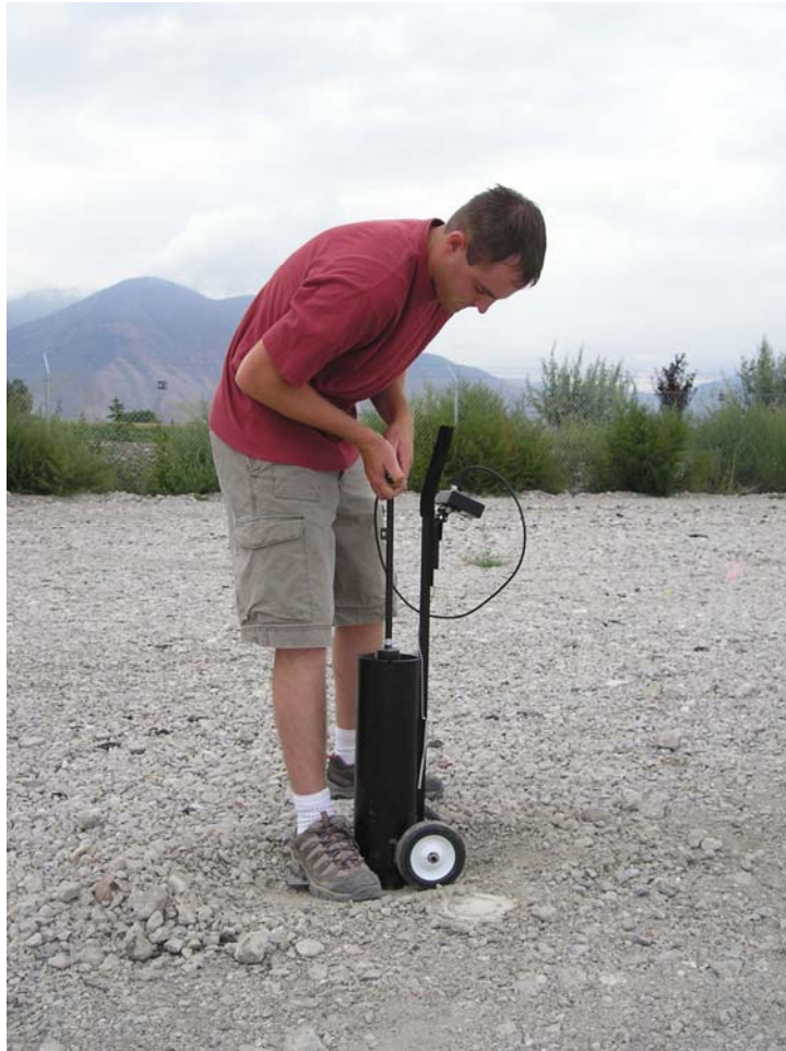
FIGURE 3-11 Heavy Clegg impact soil tester.
