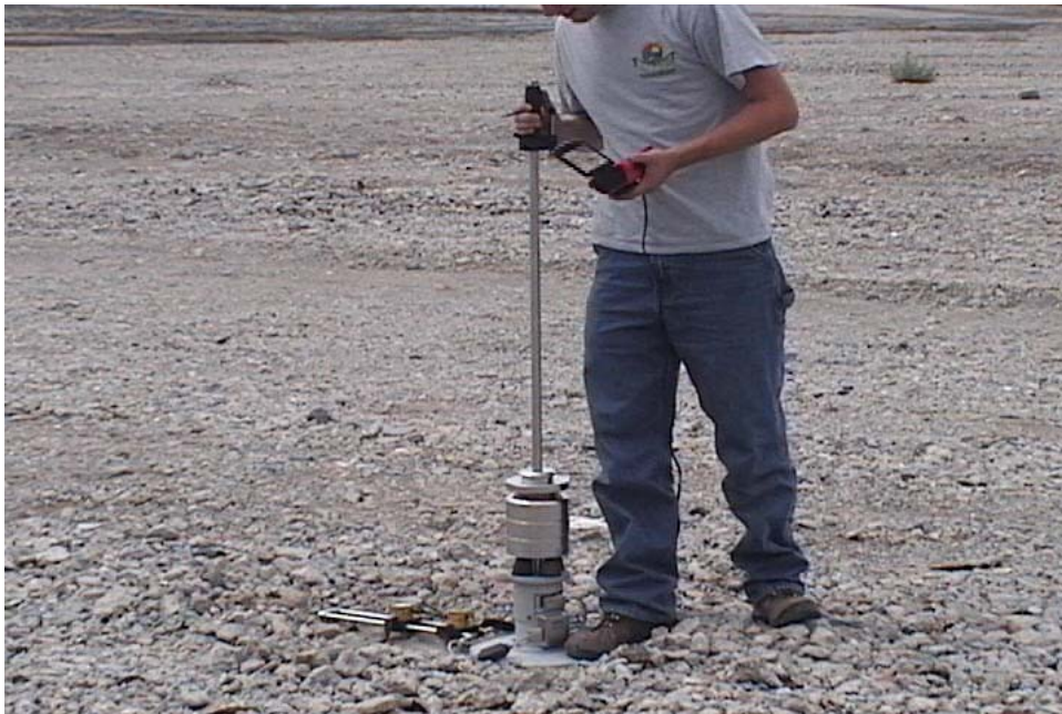
FIGURE 3-13 Portable falling-weight deflectometer.
