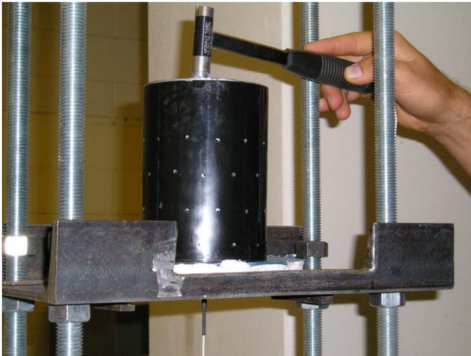
FIGURE 3-5 Specimen stand for stiffness testing.
