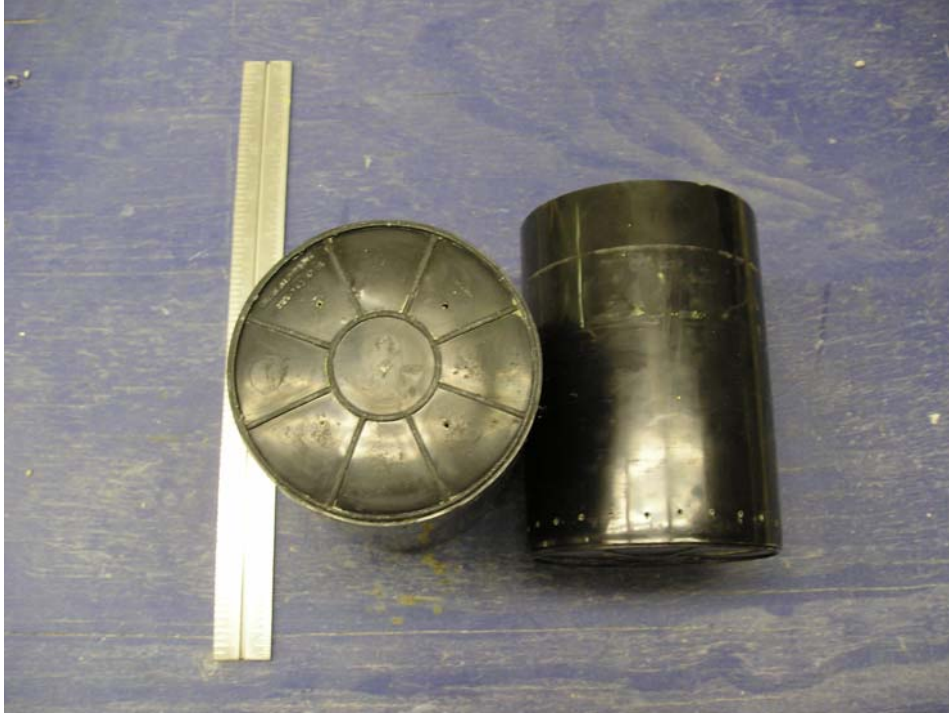
FIGURE 3-8 Specimen mold for tube suction test.
