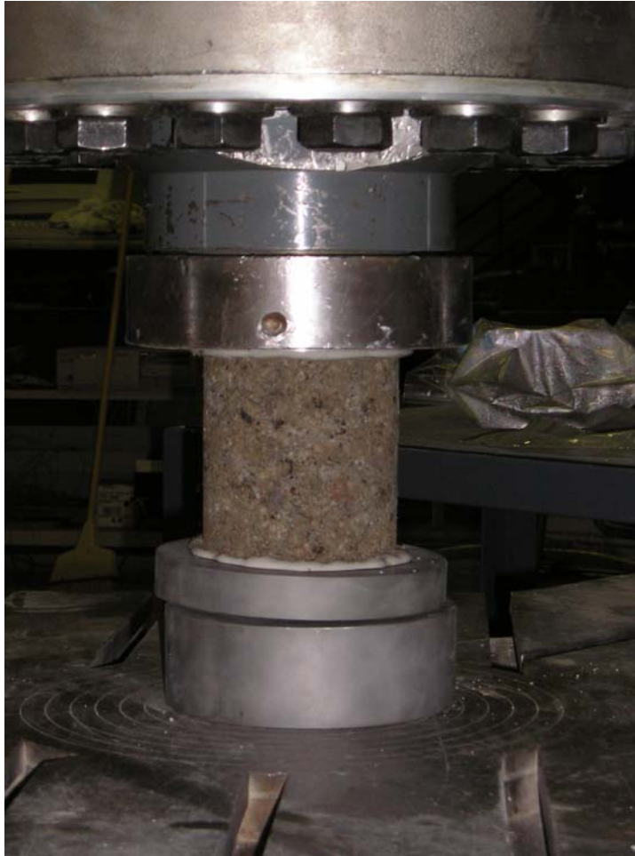
FIGURE 3-3 Unconfined compressive strength test using floating head.
