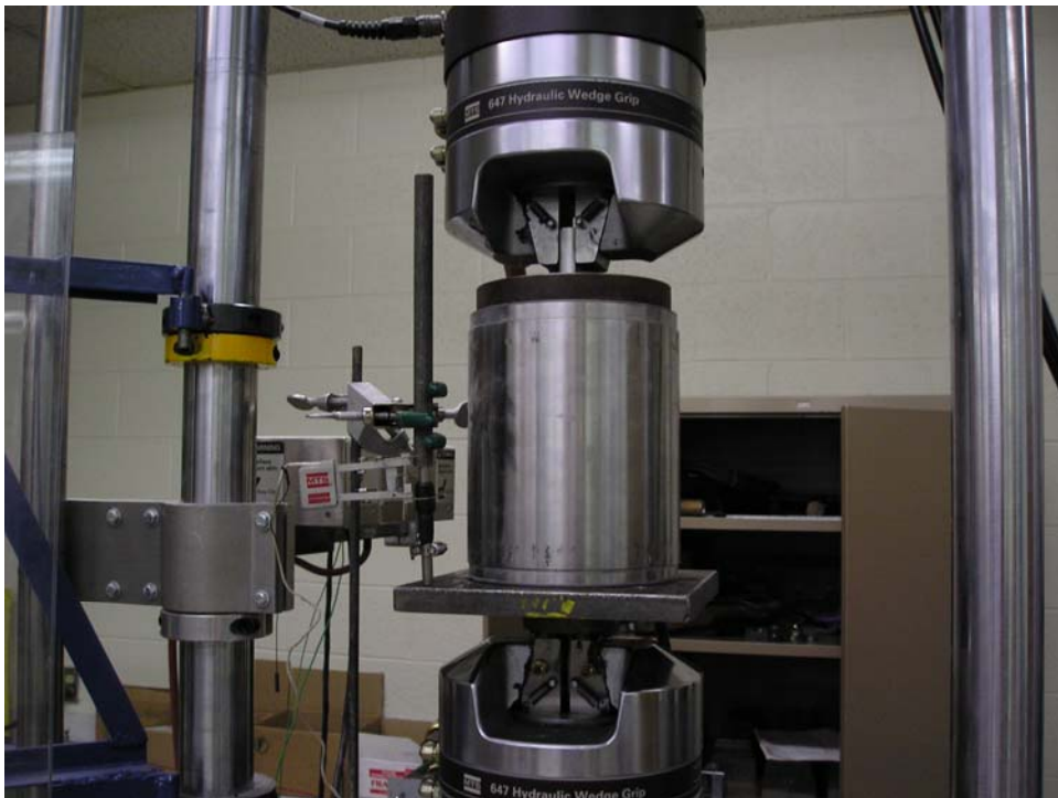
FIGURE 3-1 California bearing ratio testing.
