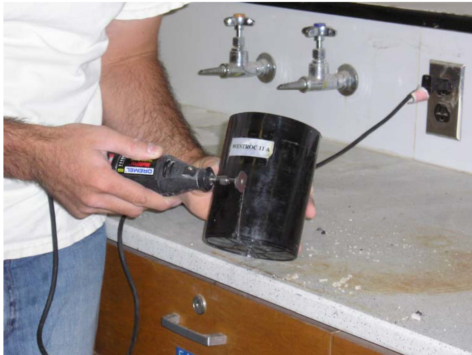
FIGURE 3-2 Removal of plastic mold.
