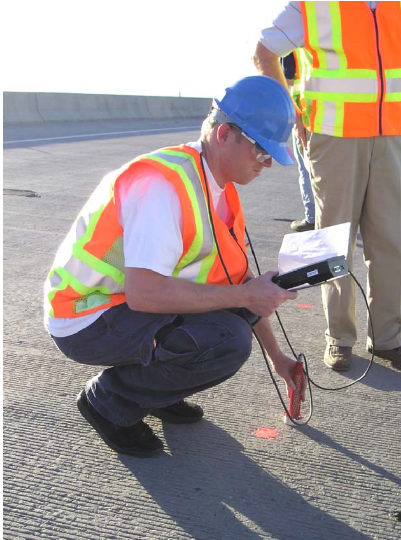
FIGURE 3.5 Measuring dielectric values.
