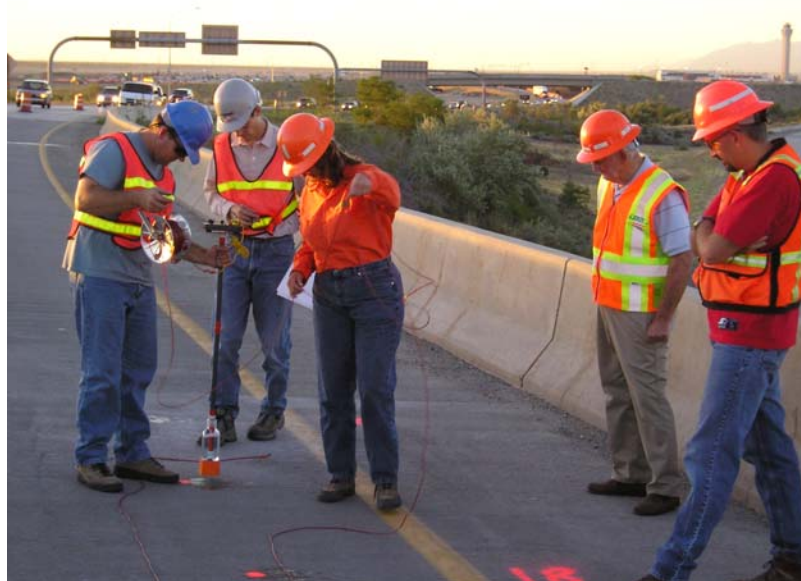
FIGURE 3.17 Obtaining half-cell potential measurements.
