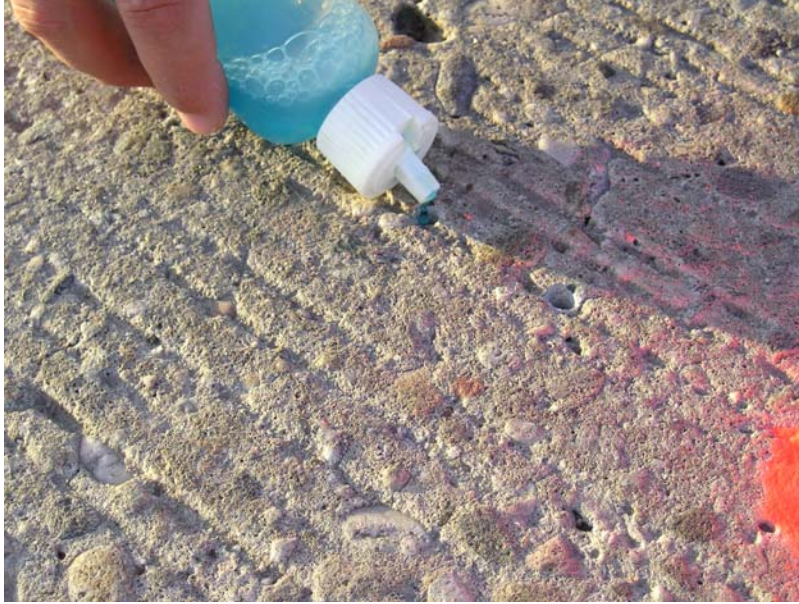
FIGURE 3.10 Placing conductive gel in test holes.
