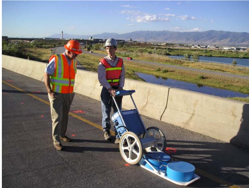
FIGURE 3.7 Ground-penetrating radar apparatus.
