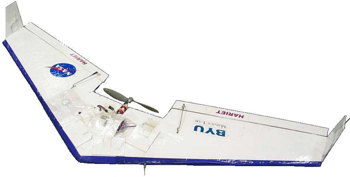
Figure 2.3: Finished UAV: Autopilot, Gimbal, GPS etc..
