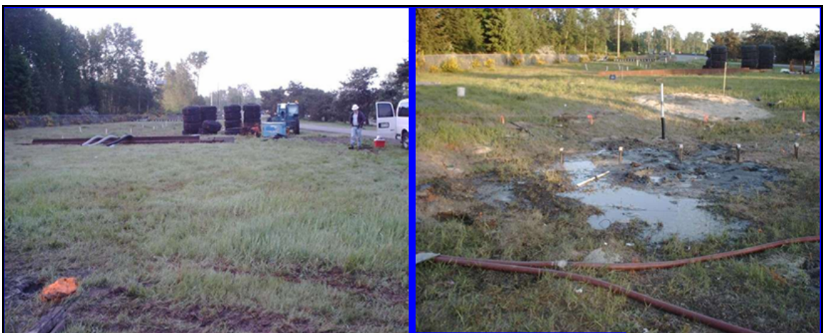
Figure 9-12 Soil Surface Before (Left) and After (Right) Blast Series 3
