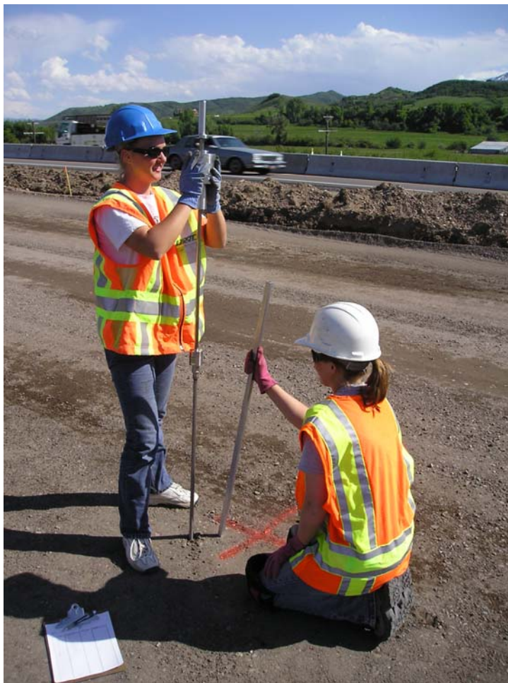
FIGURE 3.11 Dynamic cone penetrometer.
