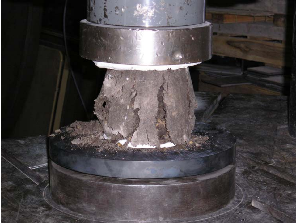
FIGURE 3.17 Splitting failure of cement-treated specimen.
