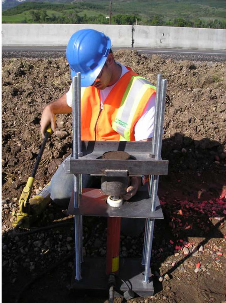
FIGURE 3.10 Extruding cement-treated specimens.
