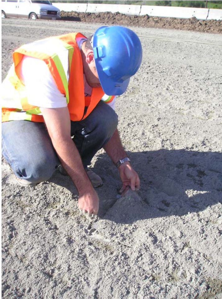
FIGURE 3.6 Retrieving cement collection sheet.
