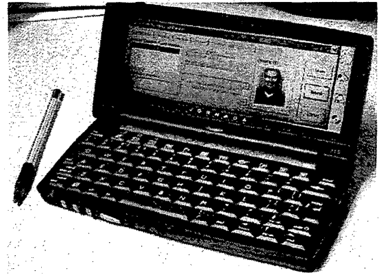
Figure 6. Handheld computer HPD based on the HP Jornada 720.
