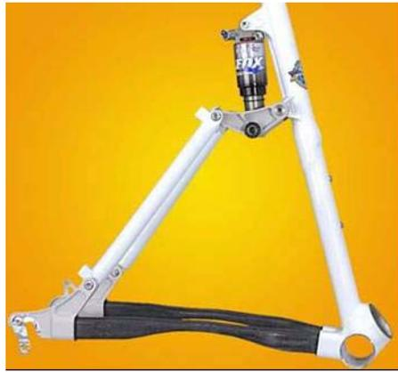
**Figure 2.14** Canondale Scalpel rear suspension ([http://www.cannondale.com/bikes/innovation/clinics/scalpel/scalpel\\_12.html](http://www.cannondale.com/bikes/innovation/clinics/scalpel/scalpel_12.html))
