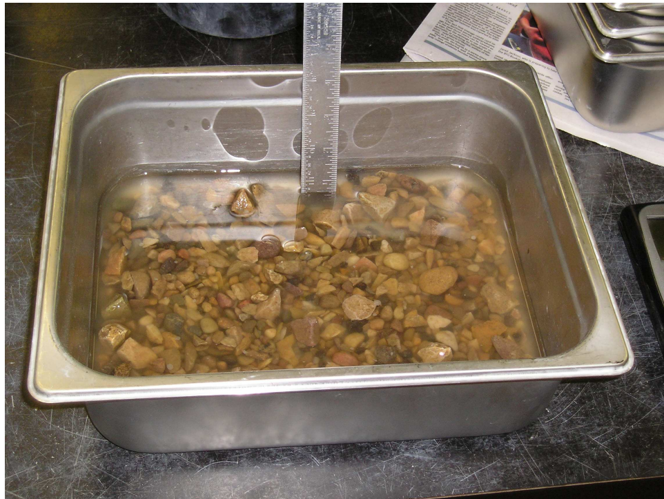
FIGURE 3.3 Soaking of coarse aggregate.
