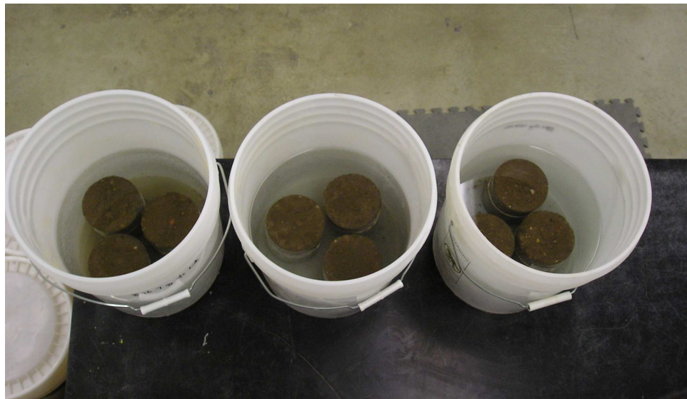
FIGURE 3.6 Soaking of UCS specimens.
