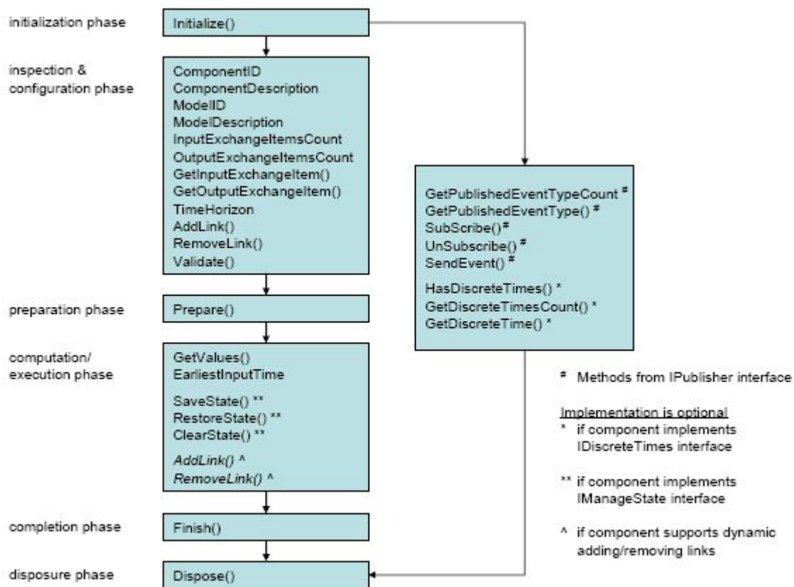
Figure 6-1 Required sequence for invoking methods in the Linkable Component [source: adopted from (Gijsbers, 2005)]
