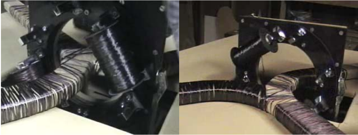
Figure 5.26 The fiber line II. Left – the spools, and hence the fiber placement (there is no special eyelet for this machine) are seen not facing the T’s intersection. Right – the spools are facing the T’s intersection.
