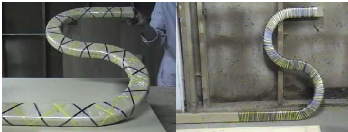
Figure 5.40 Helical and hoop windings, respectively.
