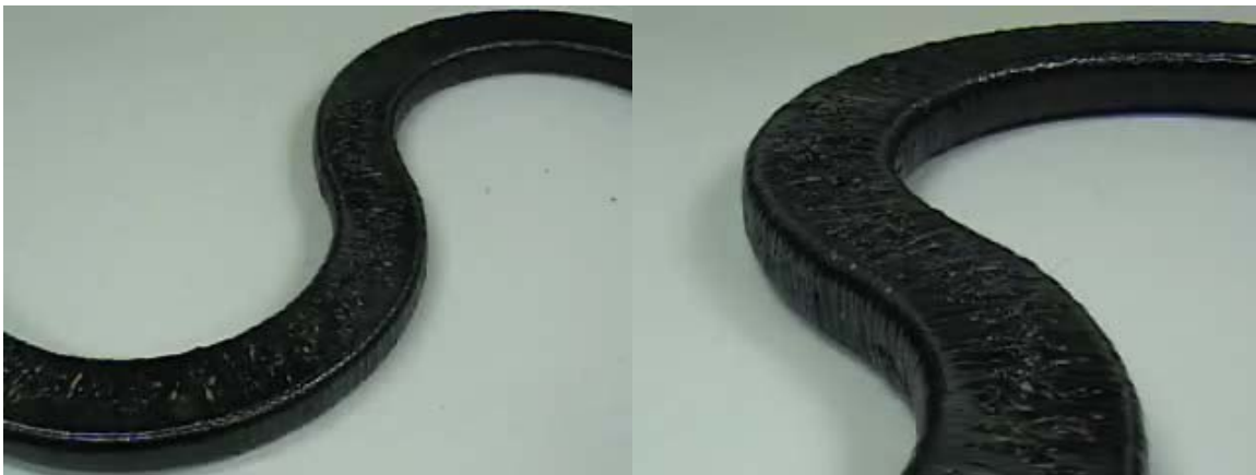
Figure 5.44 S detail. The valleys can be seen down the center of the top surface.
