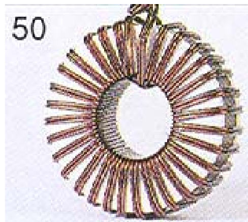
Figure 2.11 A 120mm transformer wound with a Ruff toroid winding head (Ruff, 2002). This toroid is a result of the winding described in Figure 2.10 above.
