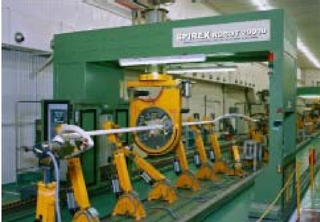
Figure 2.14 Winding mica tape on Roebel bars with a robotic system (Tari, Yoshida, Sekito, Allison, Breutsch, & Lutz, 2001).
