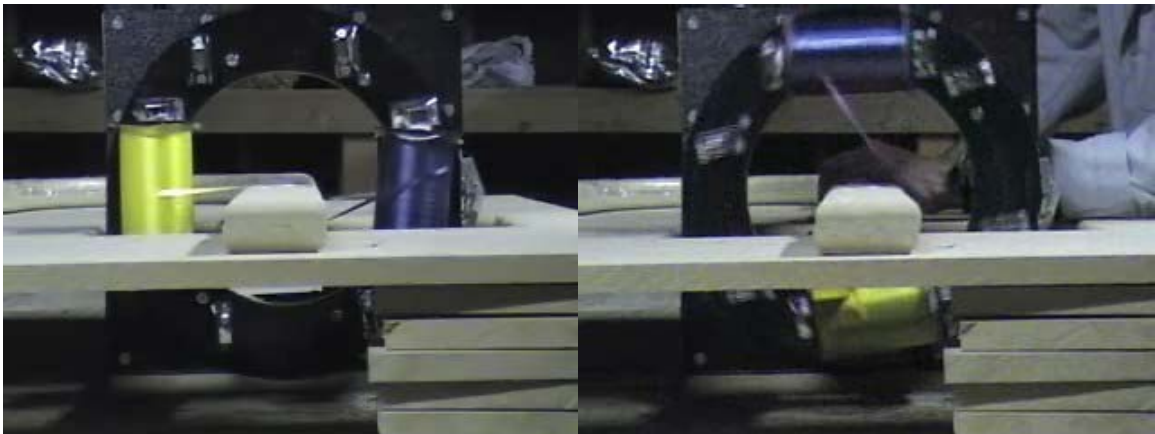
Figure 5.6 With the machine closed, the shuttle spins independently of the race.
