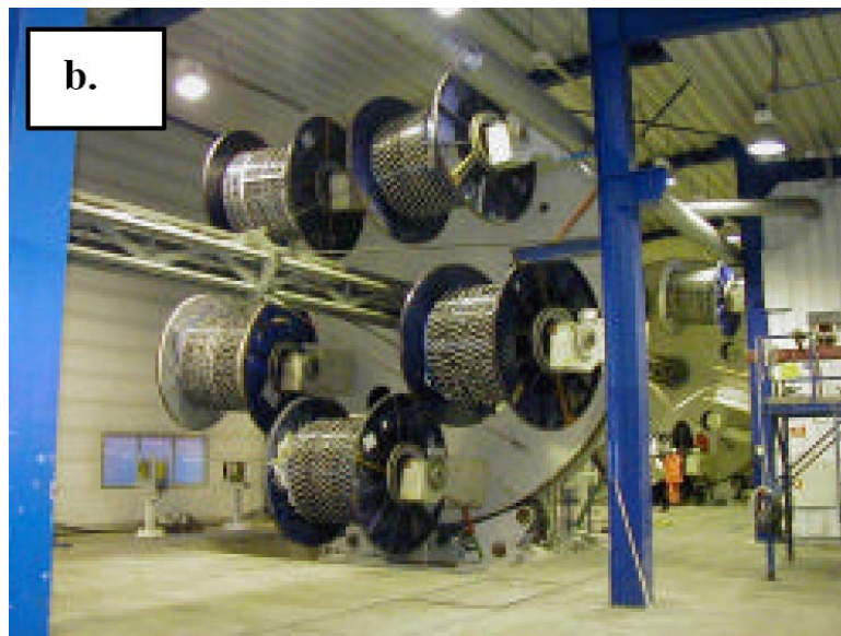
Figure 1.4 A machine making CompTether™ tendons which are used to tether Tension Leg Platforms to the ocean floor. Carbon fiber rods are wound helically around these very long tendons (DeepWater, 2004).
