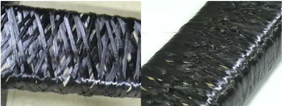
Figure 5.37 Before and after curing, respectively.
