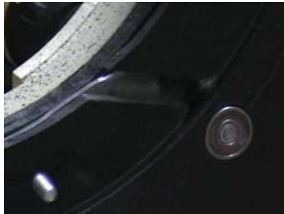
Figure 5.49 The gap. The round circle is a bearing that holds the end of the drive shaft.
