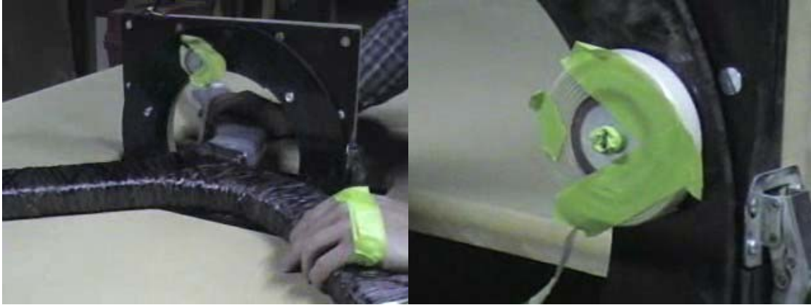
Figure 5.54 Without the spool holders the Lotus machine's working profile is smaller, giving the system more flexibility.
