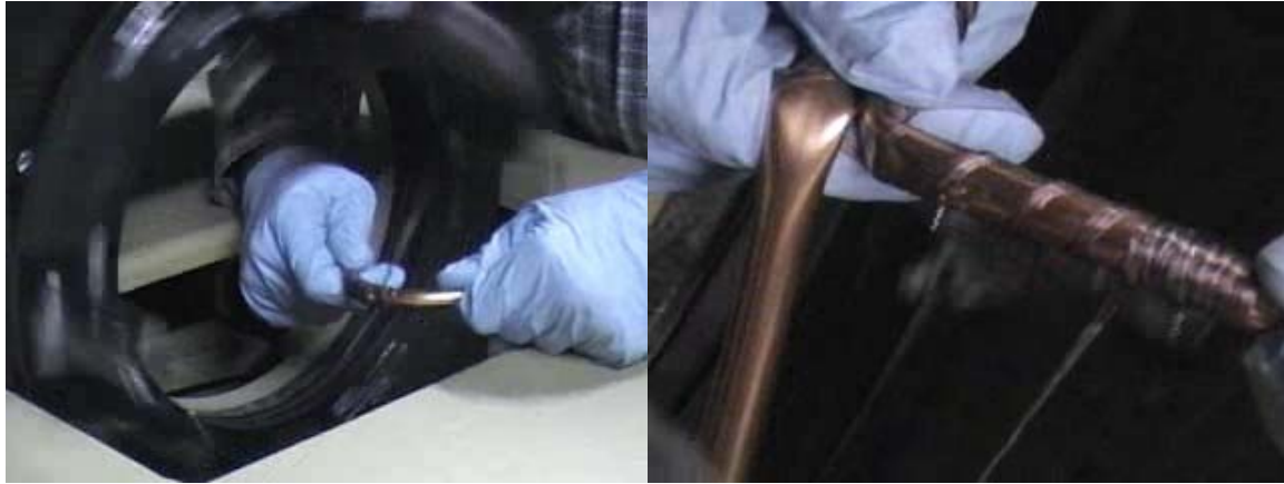
Figure 5.47 Detail of making small Lotus shapes. Left – notice the operator’s hands hold the small mandrel from both sides of the machine. Right – detail of winding a 3D Lotus T shape.
