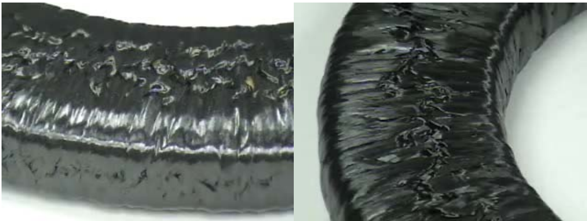
Figure 5.21 Detailed images of the O shape after curing.
