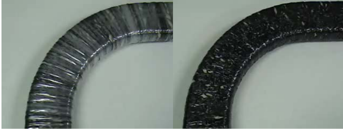
Figure 5.14 The finished L shape a) with shrink-tape, and b) without.
