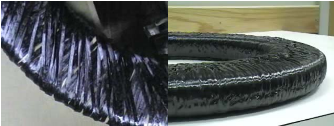
Figure 5.20 a) Hoop windings can be seen underneath the helical windings, and b) detail of the cured O shape.
