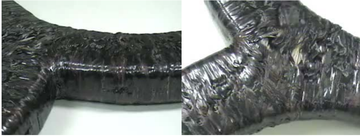
Figure 5.31 Detail of the intersection. Left – a small “valley” can be seen on the vertical face of the T. This valley is much smaller than those on the top. The finish on the side is fairly good otherwise. Right – notice a gap in the center of the intersection. This may have been caused by the operator trying to cover just one side (the other side).
