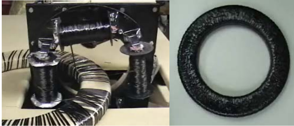
Figure 5.18 O shape setup a) An O shape being wound with 4 spools, notice these are hoop windings, and b) after curing.
