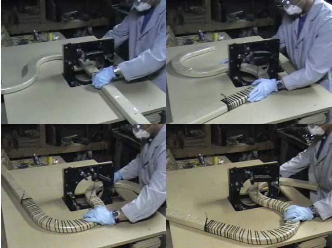
Figure 5.41 Progression of the S shape through the machine.
