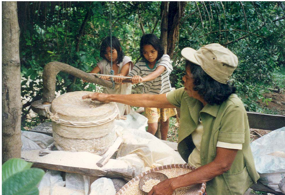
Figure 2.1 Hand-powered corn mill in the Philippines. It’s a center-less wheel. This photo was taken by the author in October 1995 in Talamban, Cebu, Philippines.
