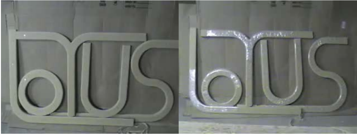
Figure 5.10 The Lotus shaped mandrels were machined from MDF and wound with tape to prevent the resin from seeping into the MDF.
