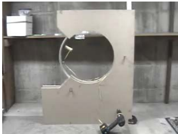
Figure 1.5 The prototype C-shaped Lotus machine used to prove the concept.
