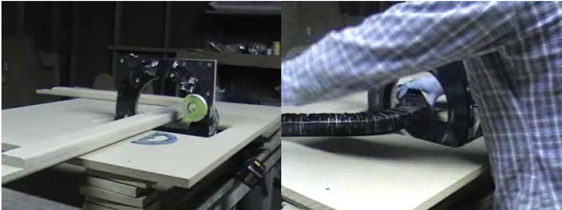
Figure 5.13 The L shape a) before being wrapped with tape, and b) being wound with prepreg carbon fiber.
