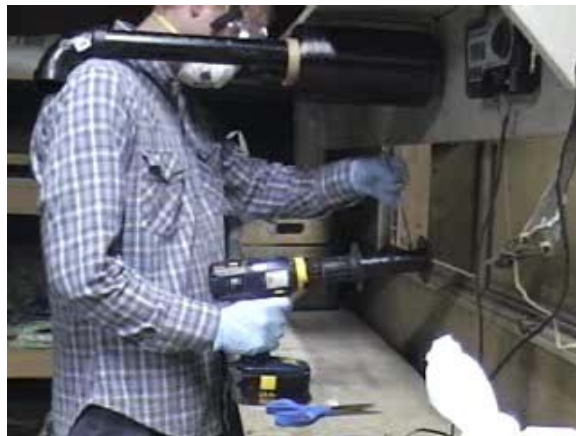
Figure 5.9 Winding a small spool with prepreg carbon fiber from a large spool.
