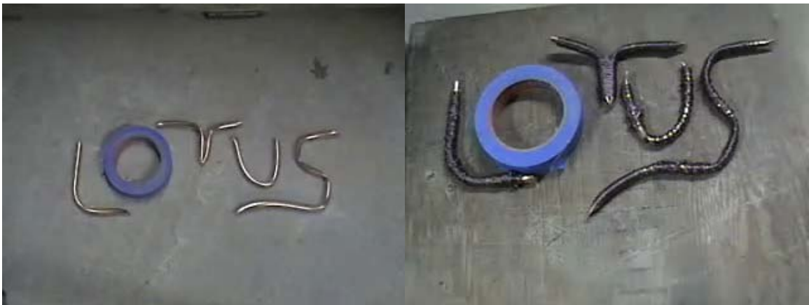
Figure 5.46 The small Lotus shapes before and after being wound. The mandrels are 3/8^{\text{th}} inch copper tubing.
