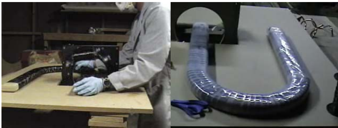
Figure 5.36 The U shape. Left – winding. Right – with heat-shrink tape.
