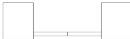
Figure 4.4 Lotus profile with work envelope center line. The small line in the center of the fiber line is where the center of the work envelope and the center of the fiber line meet. This small line is referred to as “the center of the work envelope”.
