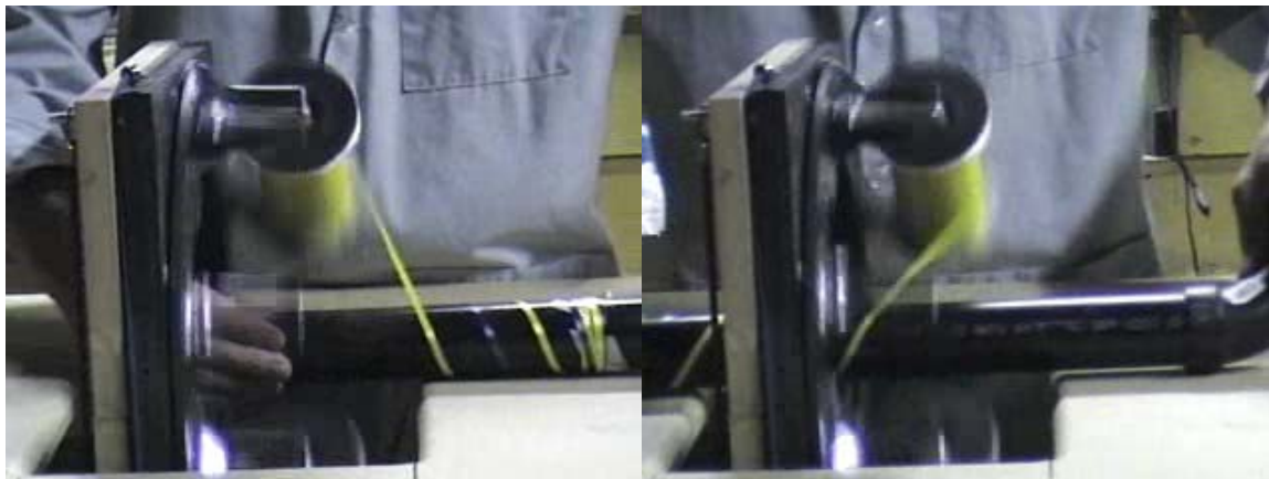
Figure 5.52 Winding drape angle.
