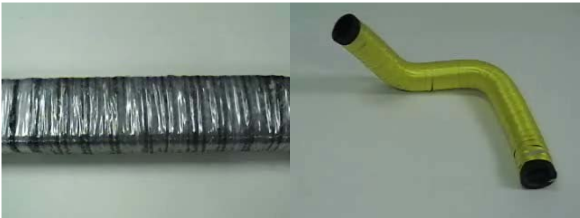
Figure 5.16 Simple and complex. a) Straight sections are easily wound with the Lotus machine, and b) simple 3D L shapes are also wound without difficulty. Notice that the tube's angles are obtuse.
