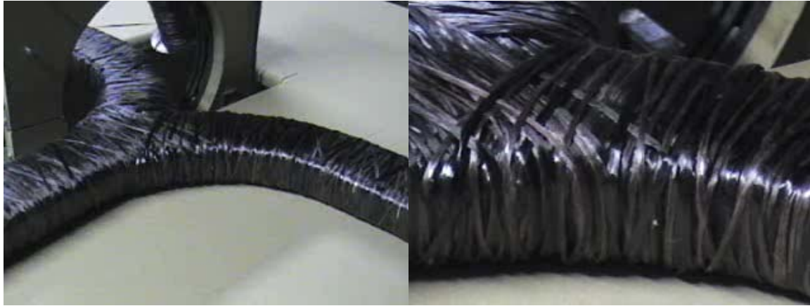
Figure 5.28 Winding up the other legs. Left – it seem there was enough stiction in the prepreg to wind up each leg quite far. Right – the overlapping of the hoop windings.
