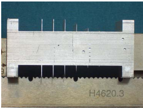
C. Top: second skim pass Bottom: rough cut only
