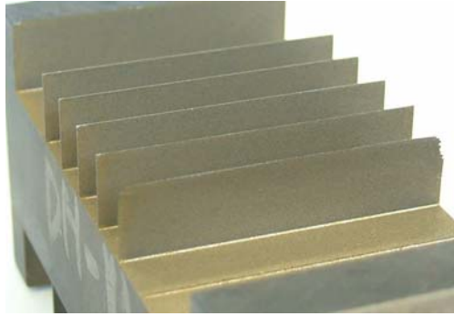
Figure 4.8 The side view of D2 heat-treated tool steel for the Rough & one skim cut
