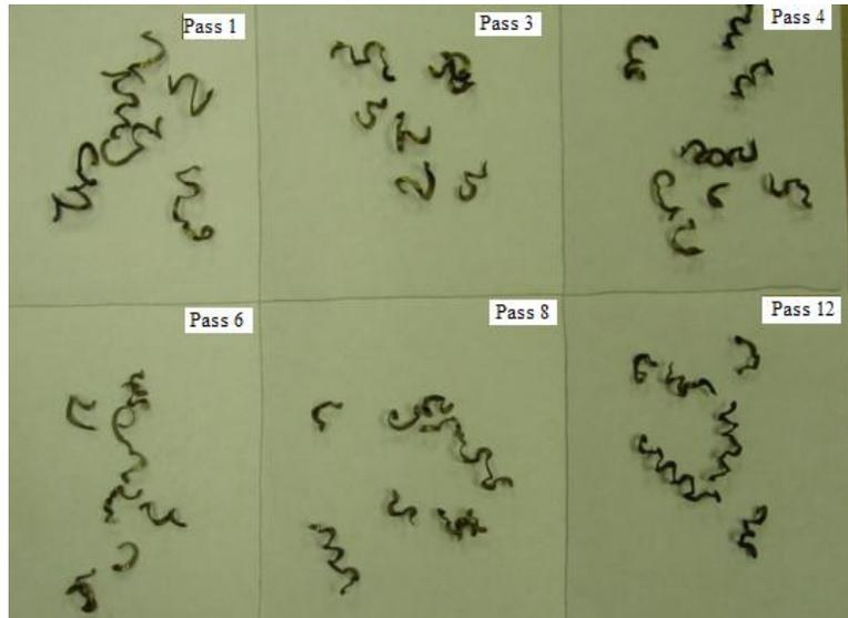
Figure D.9 Chip images for the 0° side rake angle cutting tool at 35 m/min.
