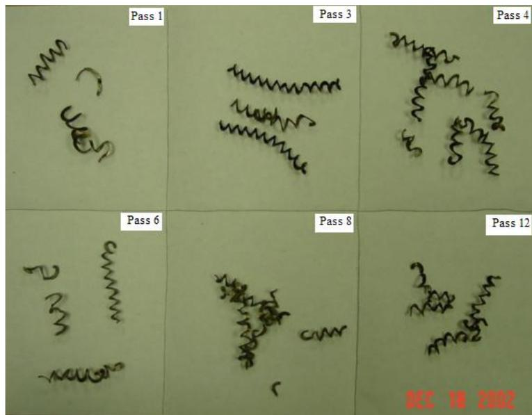
Figure D.10 Chip images for the 5° side rake angle cutting tool at 35 m/min.
