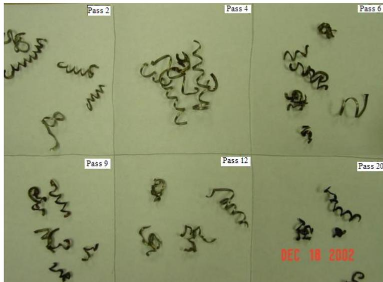
Figure D.6 Chip images for the 5° side rake angle cutting tool at 30 m/min.
