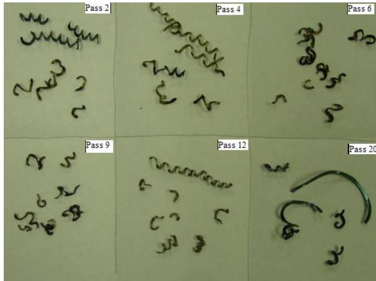
Figure D.5 Chip images for the 0° side rake angle cutting tool at 30 m/min.
