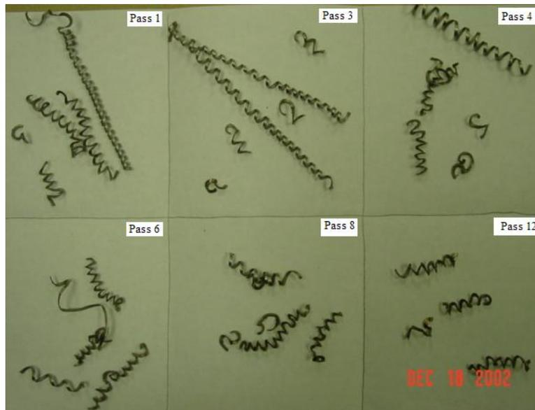
Figure D.2 Chip images for the  $5^\circ$  side rake angle cutting tool at 25 m/min.
