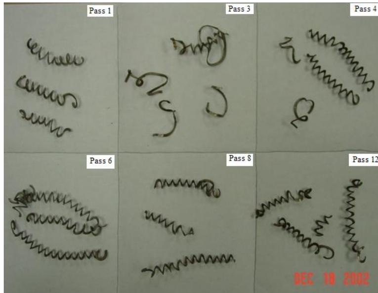
Figure D.11 Chip images for the 10° side rake angle cutting tool at 35 m/min.
