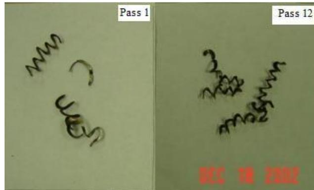
**Figure 4.11 Chip images from the first and last sampling for the 5° side rake tool at 35 m/min.**
