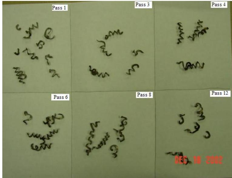
Figure D.1 Chip images for the  $0^\circ$  side rake angle cutting tool at 25 m/min.
