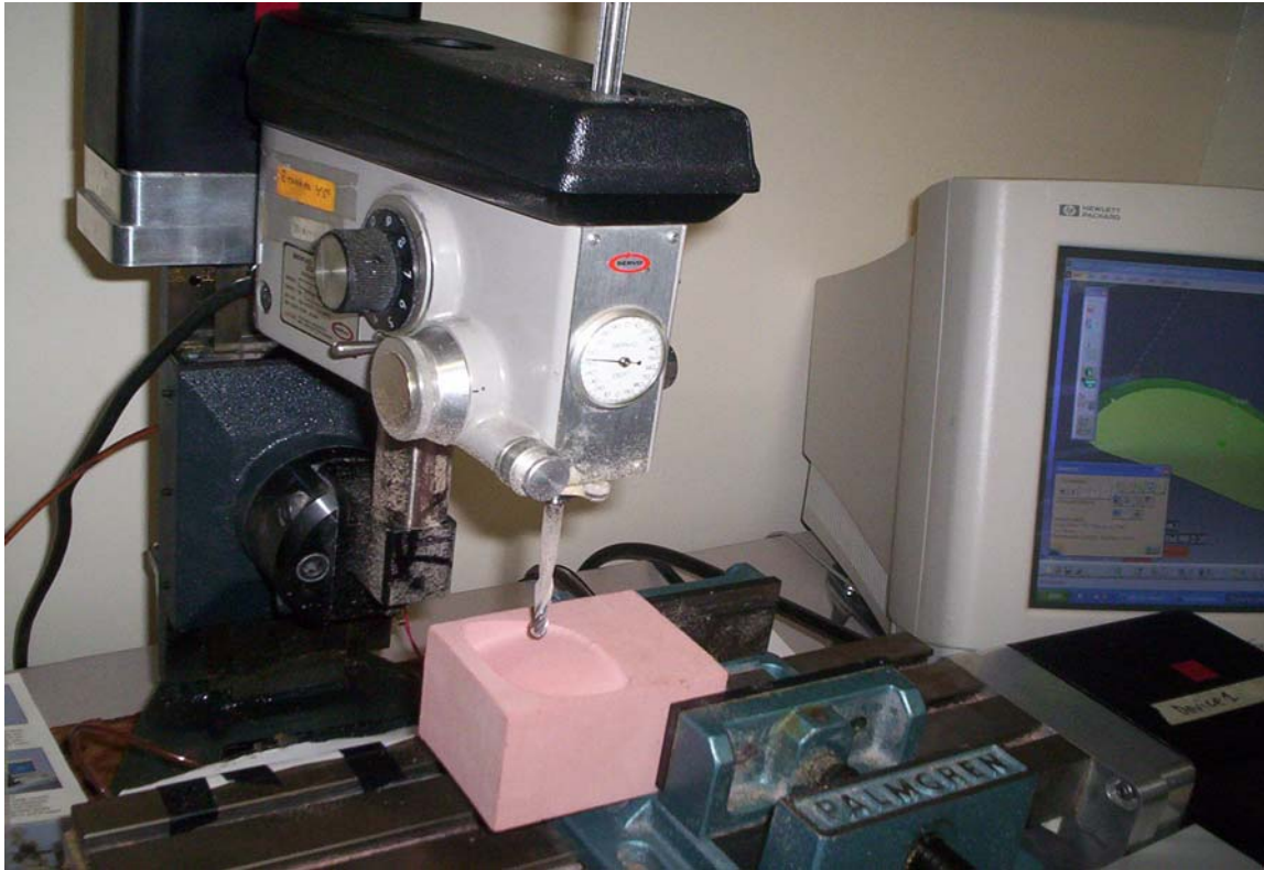
Fig. 6.7 Direct machining a car headlight on the three-axis mill
