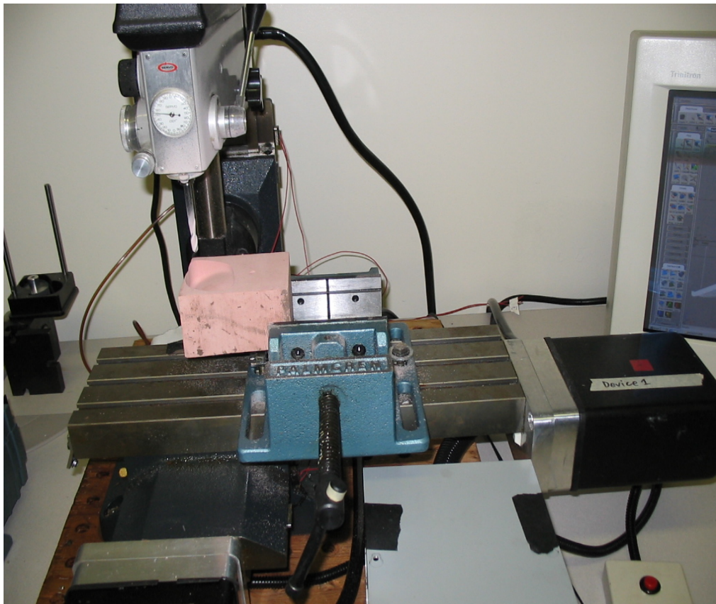
Fig. 5.1 Three-axis tabletop mill
