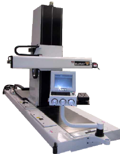
Fig. 5.2 Five-axis full-size Tarus mill
