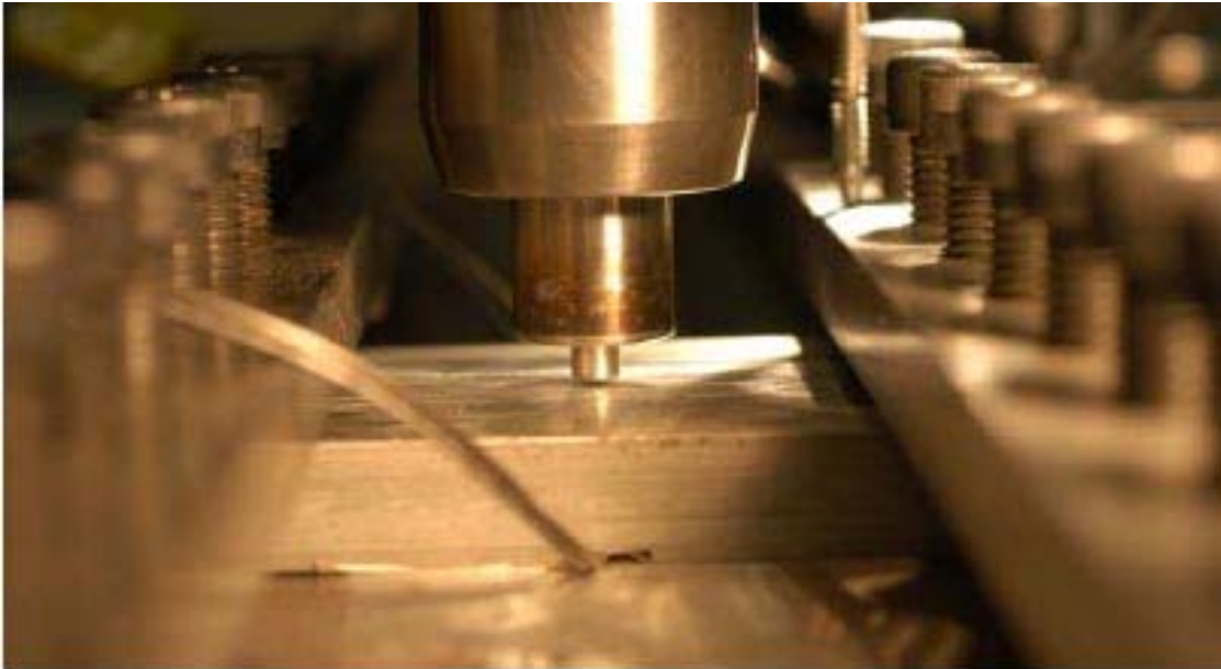
Figure 17: The FSW setup just prior to the start of an experiment.
