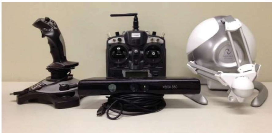
Figure 3. Navigation devices: joystick, radio control, movement and haptic sensors.
