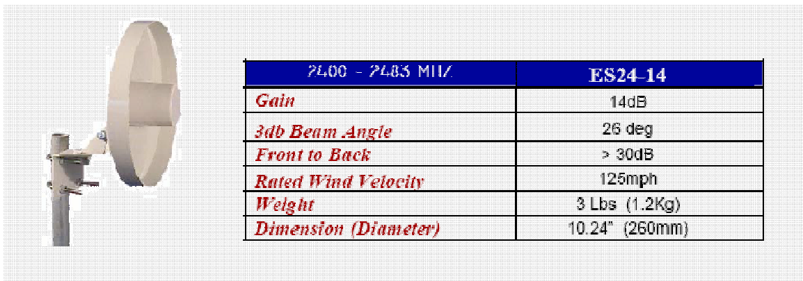
Figure 2-23 Pacific Wireless Echo Backfire specifications (PacWireless Echo 2004)
