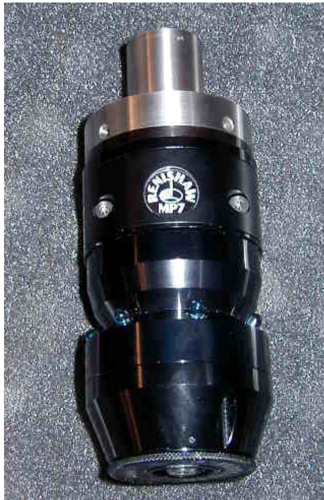
Figure 3-26 The adapter for the Sugino V9 is mounted to the top of the MP7 probe.
