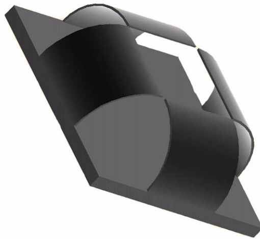
Figure 8.6 Initially-Curved Beam Configuration.
