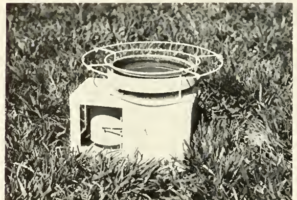
Fig. 5. Evaporimeter for daily measurement of potential evaporation.
