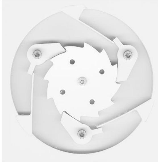
**Figure 7-1** A traditional rigid-body ratchet and pawl clutch.
