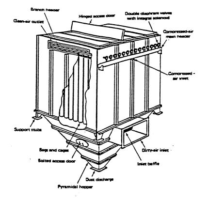
Pulse jet cleaning-parameters.
