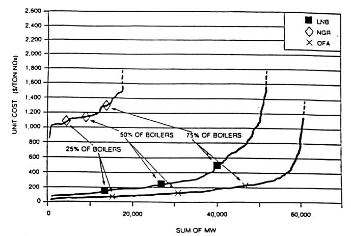
LNB = Low Nox Burners NGR = Natural Gas Burners OFA = Overfire Air
