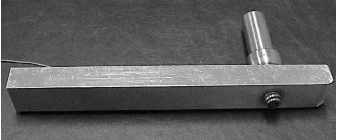
Figure 16- Typical FSW tool for polymers.
