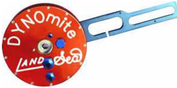
The DYNomite Land and Seas dynamometer was used to gather all clutch test data. The Dynamite consist of a 9" toroid water break absorber, electronic torque arm transducer, data wiring harness, and data acquisition computer. The dynamometer uses a manual water brake load valve to apply a torque load to the output shaft, while the torque arm transducer records the transmitted torque from the engine.
