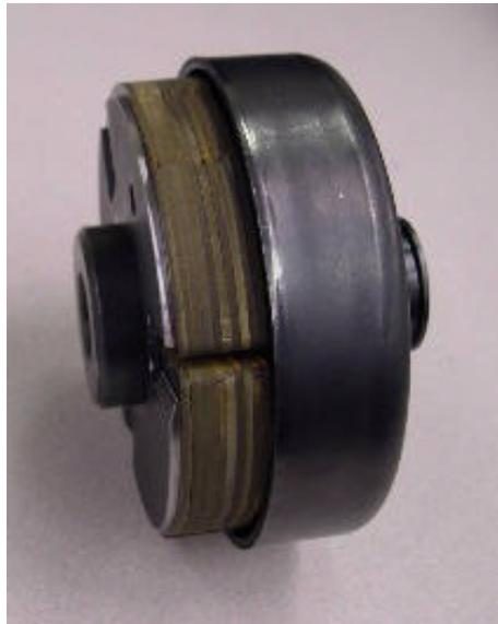
**Figure 6.6** MFOA clutch assembled into a Comet drum. The clutch consists of 10 layers of spring steel: each 0.062" thick.
